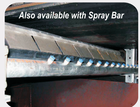
Blade Cartridge for easy blade change out.
