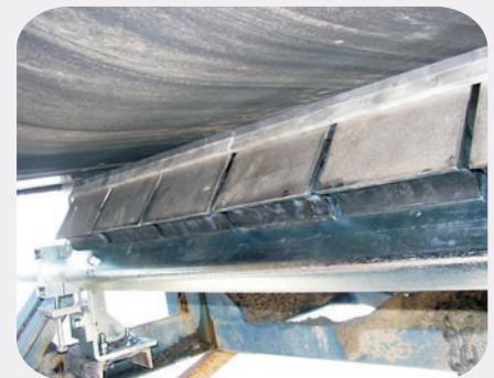
Razor-Back with V-tips installed on this coal handling conveyor at a major coal-fired power plant.
