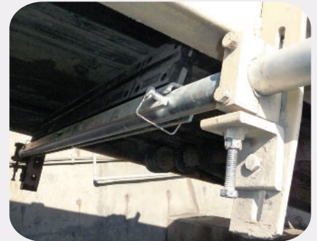
Tru-Trac Toro secondary belt cleaner installed on the primary belt off the main crusher.
