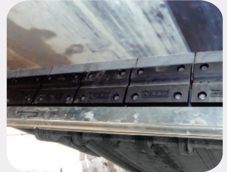
Tru-Trac Toro secondary belt cleaner installed on the primary belt off the main crusher.
